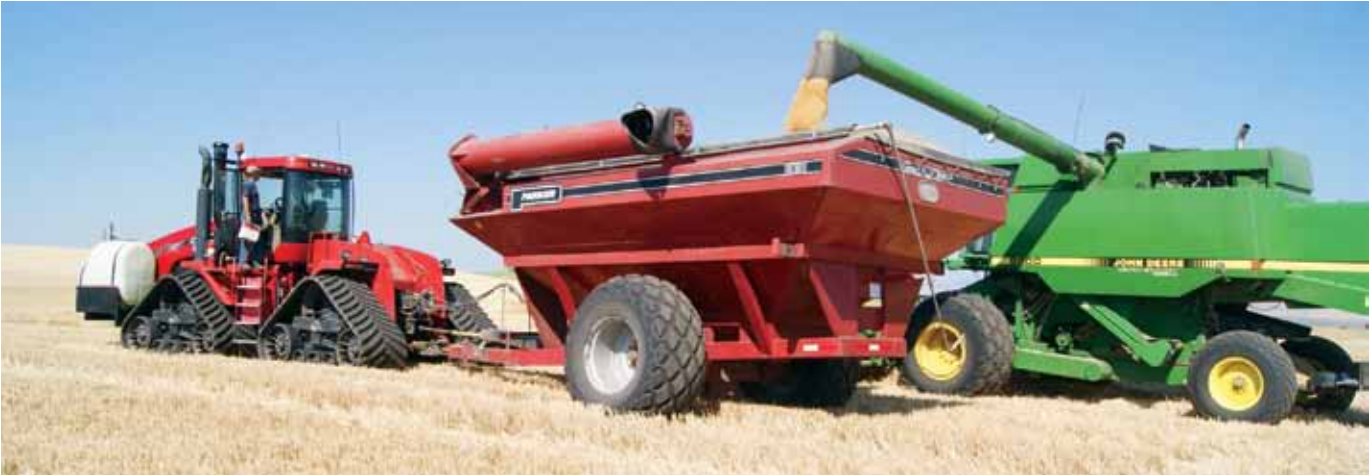
Combine unloading in bankout wagon during harvest on a farm east of Genesee, Idaho. Photo by Hilary Donlon.
