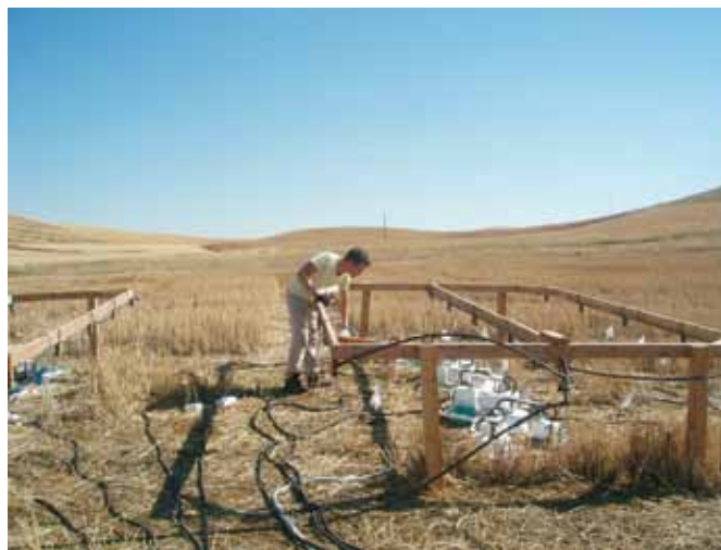
Figure 1. Dr. Kirill Kostyanovsky applies water and nitrogen treatments to no-till winter wheat stubble. Automated static chambers monitor subsequent greenhouse gas emissions on micro-plots. Photo by Dave Huggins.
