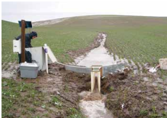
Figure 1. Water quality monitoring at the outlet of the 14-ha Idaho conventional tillage site. Photo by Erin Brooks.
