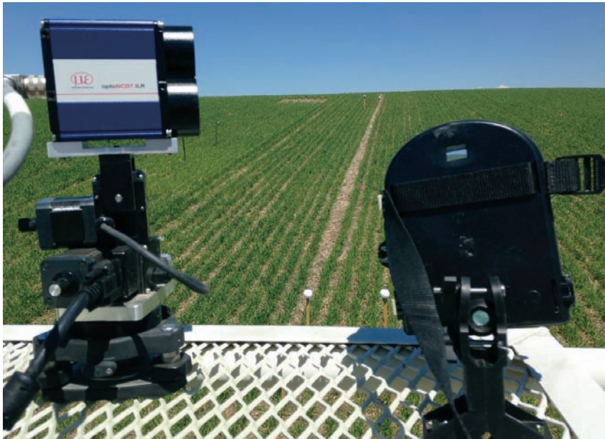
Figure 2. Time-lapse digital camera (on the right) mounted to monitor spring wheat throughout the growing season. Photo by Jyoti Jennewein.
