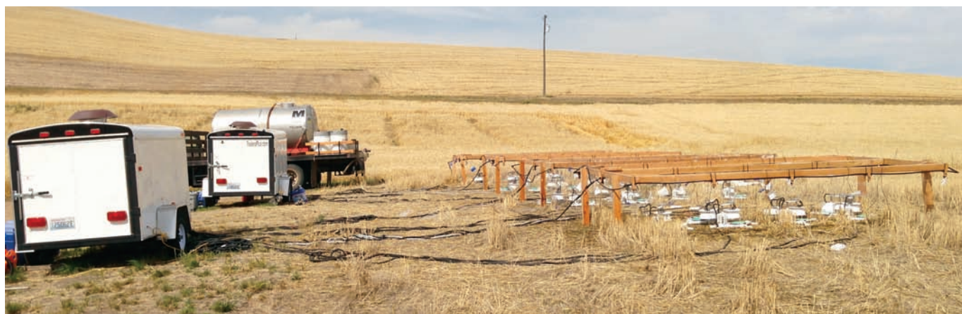
Automated static chambers monitor greenhouse gas emissions on microplots for a study designed to help predict sources of nitrous oxide emissions at different moisture levels. Photo by Kirill Kostyanovsky.
