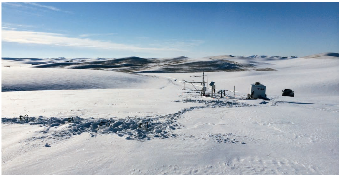
Snow removal from automatic static chambers at the long-term nitrous oxide and carbon dioxide monitoring site. Photo by Sarah Waldo.
