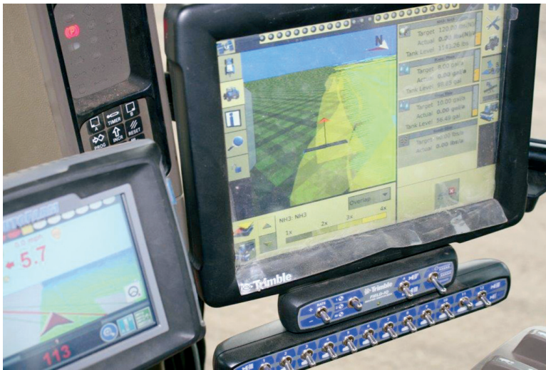
Figure 2. An example of precision agriculture software used in the field. The Trimble FmX controller (screen on right) can independently control the application rate of up to four products. Raven Envizio Pro (smaller screen on left) carries out auto-steering and provides guidance. Photo by Guy Swanson.
