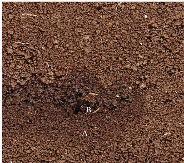
Figure 48: In-situ image of color change (A) surrounding the site of urea dissolution (B).
